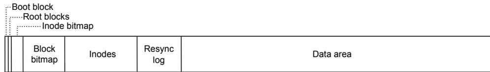
Fig. 3: High-level overview of the TwinFS on-device layout. The root, inode, and bitmap blocks are metadata and thus protected. The data area contains both protected and unprotected data blocks, as well as indirect blocks, which are metadata and thus protected. The resynchronization log is described in Sec. V-C.
