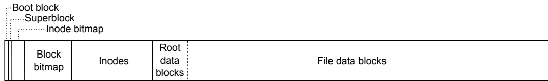
Figure 2: High-level overview of the on-disk layout used by the physical layer prototype.
