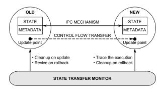
Figure 1: The state transfer process.
