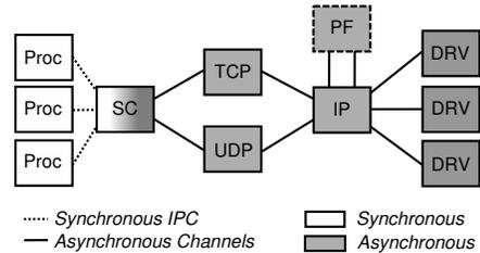
Figure 1: Design of the NewtOS network stack
