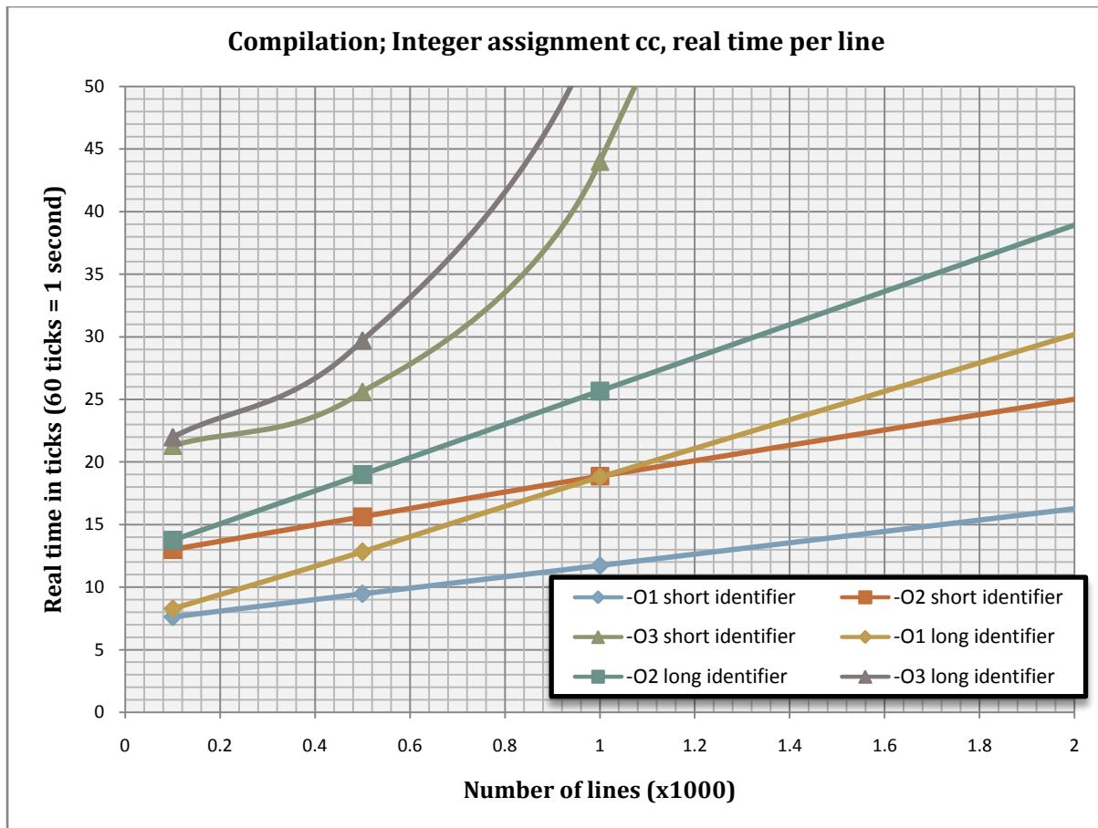
Figure 12 - Compilation real time per line, integer assignment cc (Pentium 2 350MHz)
