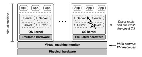
**Figure 6.3:** Full virtualization cannot isolate individual drivers. Although each virtual machine runs in isolation, a single driver fault in a guest OS can still take down an entire virtual machine.
