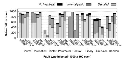
Figure 5.4: Number of driver failures and failure reasons for 4 network-device drivers and 8 fault types. For each driver and fault type we conducted 1000 SWIFI trials injecting 100 faults each.
