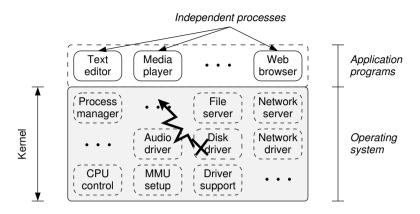
**Figure 1.3:** A monolithic design runs the entire OS in the kernel without protection barriers between the OS modules. A single driver fault can potentially crash the entire OS.
