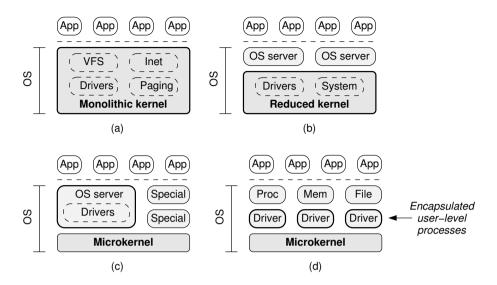
**Figure 6.7:** Granularity of process encapsulation over the years: (a) monolithic design, 1970s, e.g. BSD UNIX; (b) reduced-kernel design, 1980s, e.g. Mach; (c) single-server design, 1990s, e.g.  $L^4$ Linux; and (d) multiserver design, 2000s, e.g. SawMill Linux and Minix 3.
