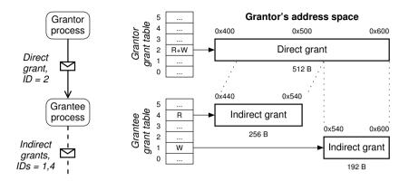
**Figure 3.5:** Hierarchical structure of memory grants. A direct grant gives access to part of the grantor's memory. An indirect grant gives access to a subpart of the *root* grantor's memory.
