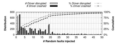
**Figure 5.6:** Number of faults needed to disrupt and crash the DP8390 driver during 100,000 random SWIFI trials. Crashes show a long tail to the right and surpass 99% only after 263 faults.
