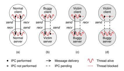
Figure 3.2: Asymmetric trust and vulnerabilities in synchronous IPC: (a) normal client-server roundtrip, (b) untrusted client blocks server, and (c) and (d) untrusted server blocks client.
