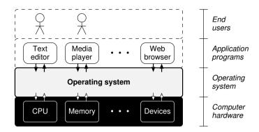
**Figure 1.1:** The fundamental role of the OS in a computer system: the OS is the lowest level of system software that controls the hardware, manages resources, and interfaces with applications.
