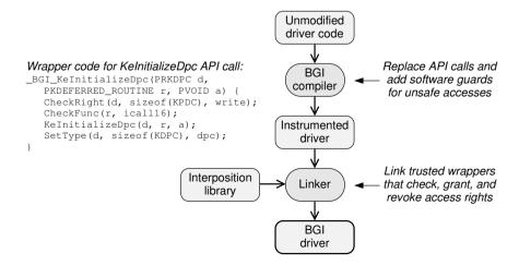
**Figure 6.2:** Software-based fault isolation in BGI. A BGI compiler replaces direct kernel API calls with wrapper calls and adds software guards before direct memory accesses and indirect calls.
