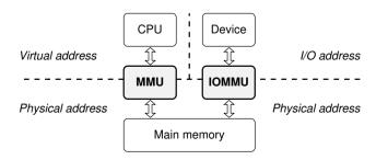
**Figure 2.7:** The MMU hardware provides memory protection for CPU-visible addresses, whereas the IOMMU hardware provides memory protection for device-visible addresses.
