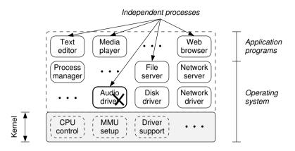
**Figure 1.4:** A multiserver design runs each server and driver as an independent, hardware-protected user process. This design prevents propagation of faults between the OS modules.
