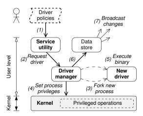
**Figure 2.5:** The administrator uses the service utility to request drivers and set isolation and recovery policies. The driver manager starts the driver and publishes its details in the data store.
