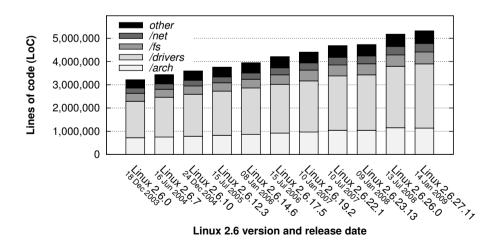
Figure 1.2: Growth of the Linux 2.6 kernel and its major subsystems in lines of executable code (excluding comments and white space) for a 5-year period with 6-month deltas.
