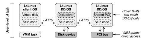
**Figure 6.4:** Paravirtualization supports safe and unmodified driver reuse by running them in their original, paravirtualized OS inside a VM. The client OS and device-driver OS (DD/OS) communicate via VM-to-VM communication primitives provided by the L4 microkernel.
