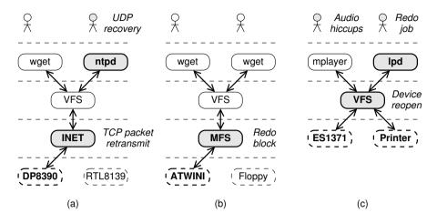
**Figure 4.6:** Components that have to be aware of driver recovery for different kinds of drivers: (a) network-device driver recovery, (b) block-device driver recovery, and (c) character-device driver recovery. A gray color indicates that a component or the end user is aware of the recovery.
