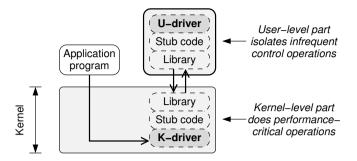
**Figure 6.8:** Split-driver architecture used by Microdrivers: applications interface with the normal kernel APIs. The kernel-level part (K-driver) calls the user-level part (U-driver) for control operations that are not performance critical.
