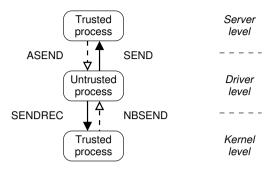
**Figure 3.6:** IPC patterns to deal with asymmetric trust. Trusted processes use asynchronous or nonblocking IPC (dashed lines) for sending to untrusted processes, which use synchronous IPC (solid lines) to prevent race conditions that may cause messages to be dropped.
