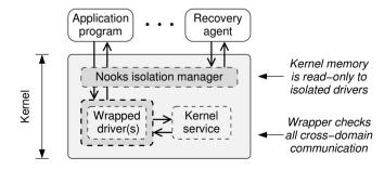
**Figure 6.1:** Hardware-enforced protection in Nooks. Nooks sets up protection domains for kernel memory and wraps drivers in a layer of protective software. If a failure is detected, the isolation manager calls a user-level recovery agent that can restart the driver.
