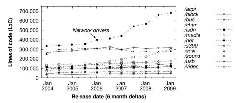
**Figure 5.21:** Linux 2.6 driver growth in lines of executable code (excluding comments and white space). Network-device drivers are both the largest and fastest-growing driver category.
