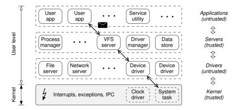
Figure 2.1: Multiserver design of the MINIX 3 OS. Each application, server, and driver runs as an independent user process. Interprocess communication (IPC) is based on message passing.
