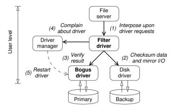
**Figure 4.7:** A filter driver between the file server and block-device driver can check for driver protocol violations. Different protection strategies based on checksumming and mirroring are supported. If an error is detected, a complaint is filed with the driver manager.
