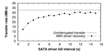
**Figure 5.17:** Throughput when using *dd* to read a 1-GB file from the hard disk with and without killing the ATWINI driver with various time intervals.
