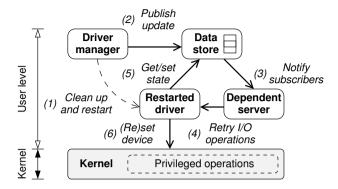
Figure 4.3: Procedure for restarting a failed device driver and reintegrating it into the system. The sequence of steps taken is shown in (roughly) clockwise order.
