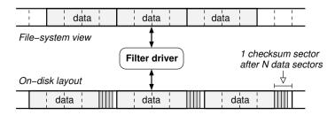
Figure 4.8: The filter driver intersperses 1 checksum sector for every N data sectors. This figure shows the file-system view and on-disk layout for N=4 checksums per checksum sector.
