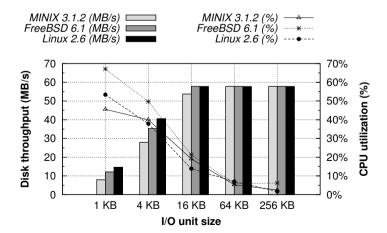
**Figure 5.15:** Cross-platform comparison of disk throughput and CPU utilization for a 2-GB read with varying I/O units from the raw block device with a sequential access pattern.
