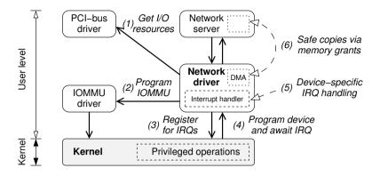
**Figure 3.8:** Interactions between an isolated network-device driver and the rest of the OS. Access to privileged resources is mediated by the PCI-bus driver, IOMMU driver, and the kernel.
