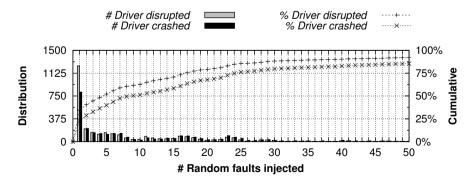
**Figure 5.7:** Number of faults needed to disrupt and crash the RTL8139 driver during 100,000 random SWIFI trials. Crashes show a long tail to the right and surpass 99% only after 282 faults.
