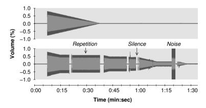
**Figure 5.10:** Normal playback of a regular audio sample (top) and playback with 10 SWIFI trials injecting 100 random faults each into the Ensoniq ES1371 PCI audio driver (bottom). Recovery is transparent to the application, but the I/O is repeatedly interrupted.
