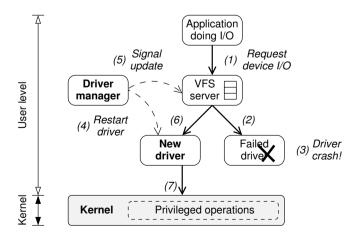
**Figure 2.8:** Basic idea underlying our failure-resilient OS. If the driver manager detects a driver failure, it looks up the driver's recovery policy, and may restart the driver and notify dependent components so that the system can continue to operate normally.
