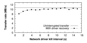
**Figure 5.16:** Throughput when using *wget* to retrieve a 512-MB file from the local network with and without repeatedly killing the Realtek RTL8139 driver with various time intervals.
