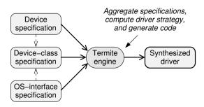
**Figure 6.6:** Formal method to synthesize drivers in Termite. Device, device-class, and OS specifications are aggregated, a driver strategy machine is computed, and driver code is generated.
